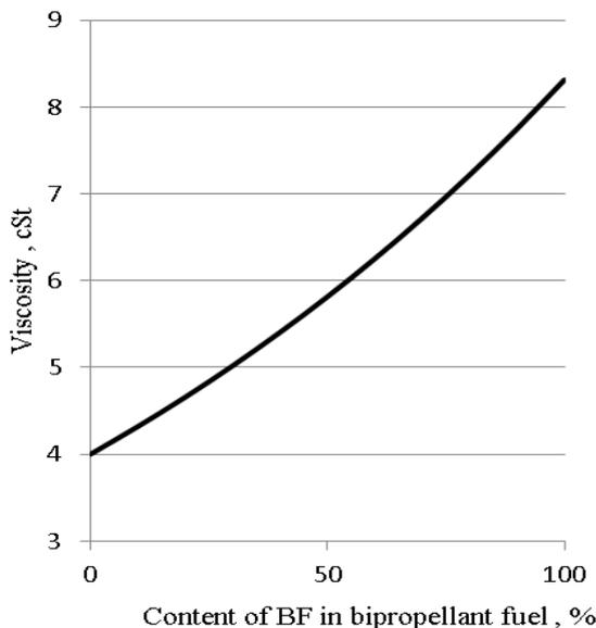
**Figure 5:** Viscosity of bipropellant fuel depending on percentage content of BF in it (calculated value)
