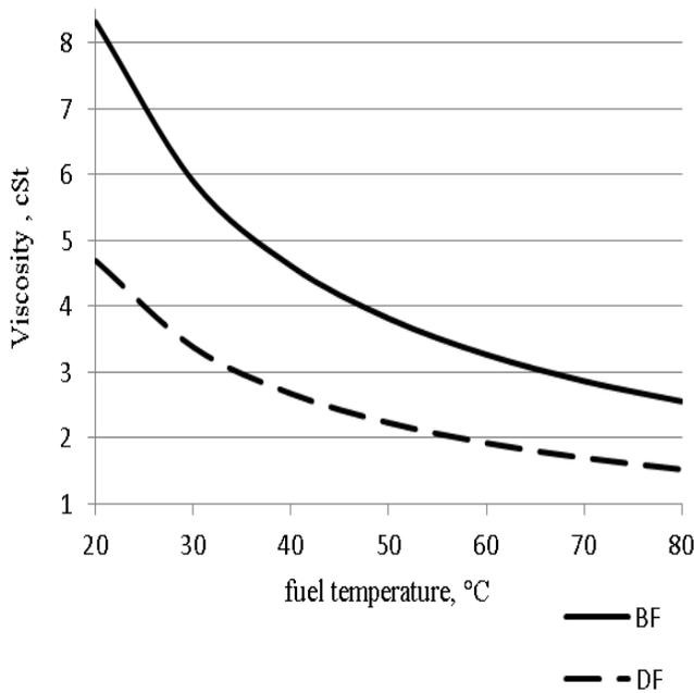
**Figure 2:** Viscosity of BF and DF depending on its temperature
