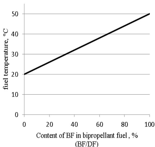
**Figure 3:** Temperature of bipropellant fuel depending on the percentage content of BF in it
