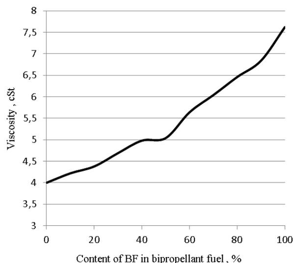
**Figure 1:** *Viscosity of bipropellant fuel depending on percentage content of BF in it*
