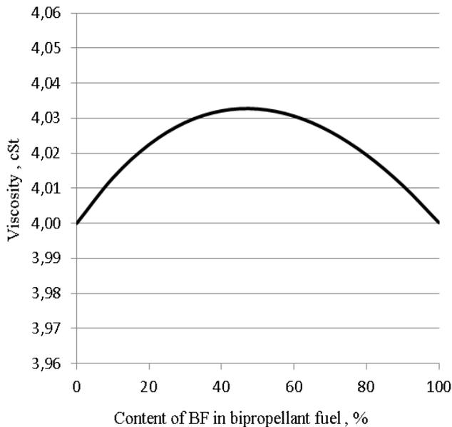
**Figure 4:** Viscosity of bipropellant fuel depending on percentage content of BF in it at fuels temperature before mixing equals: DF - 20°C, BF – 47,3 °C
